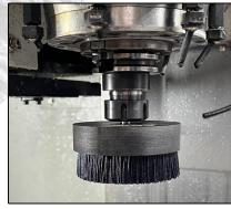
**Abtex In-Machine Deburring** System - Designed to become an integral part in most machining centers, bringing unimaginable efficiency to any manufacturing operation.
