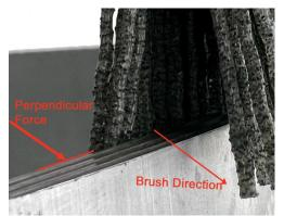
How It Works - The abrasive filament strikes the part at a perpendicular angle. The filaments are forced up and over the burrs and their cutting energy is transferred directly to where it's needed. The abrasive filament is more efficient to use rather than other deburring methods because of its self-sharpening capabilities. Any Abtex solution starts with abrasive filament material, grit, size and several other options which also allow Abtex to engineer custom designed abrasive filament brushes.
