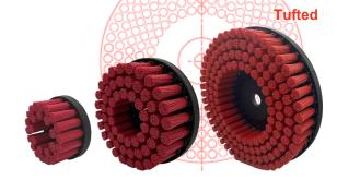
V-Tuft Abrasive Filament Brush - Ideal for more aggressive applications. The filaments are packed tighter together to prevent the filament from conforming around the burr. This style of brush is ideal for heavier metals like steel, requiring sharp edge removal, or, well attached burrs on aluminum, powdered metal, or fine-blanked parts.
